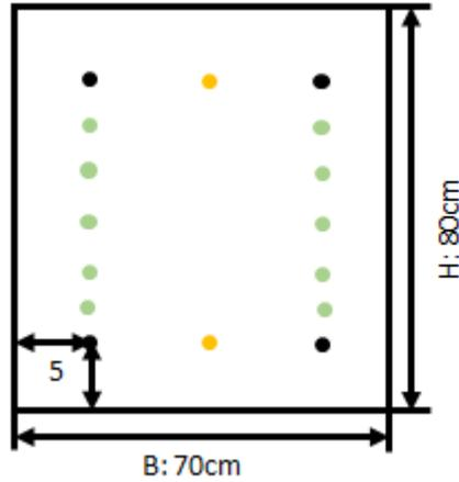
**Fig. 1** example of parametrized RC section; B for width, H for height, yellow dots for width-span rebar, and green dots for height-span rebar
