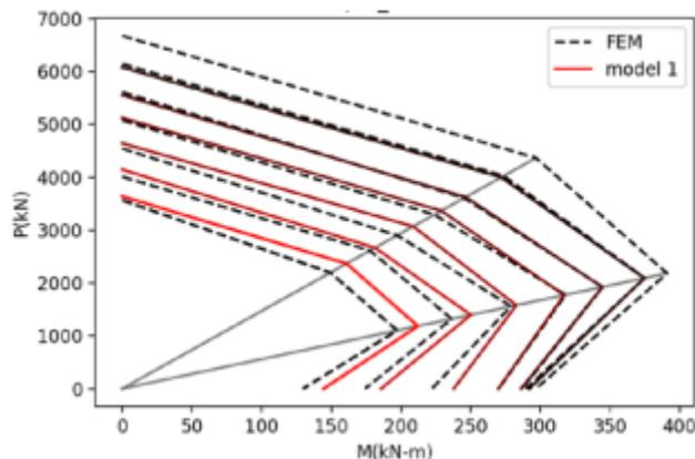
Fig. 4 example of P-M interaction diagram reconstructed (B=40, H=40, BN=6, HN=2)
