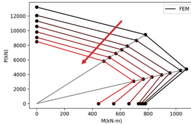
**Fig. 2** Description for 4 points reduced P-M interaction diagram of a RC section with varying fire exposure time.
